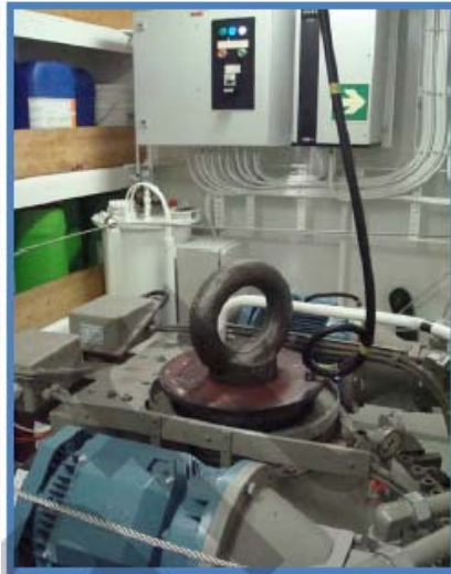
Figure 23 VFD Controlled Steering Gear
