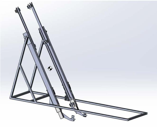
Figure 2.10: Frame for vertical conveyor.
