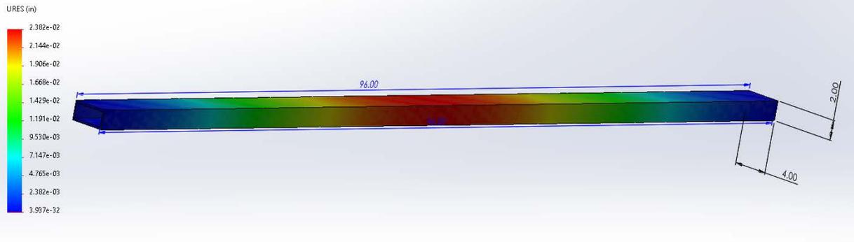
Figure 2.9 Aluminum rectangular tubing, with a maximum deformation of 0.02"
