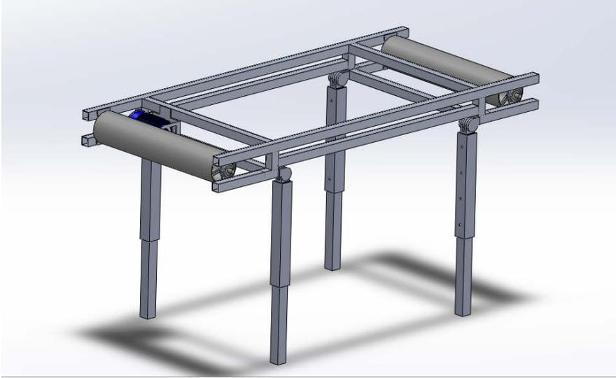
Figure 3.2: Modular conveyor sections with legs extended
