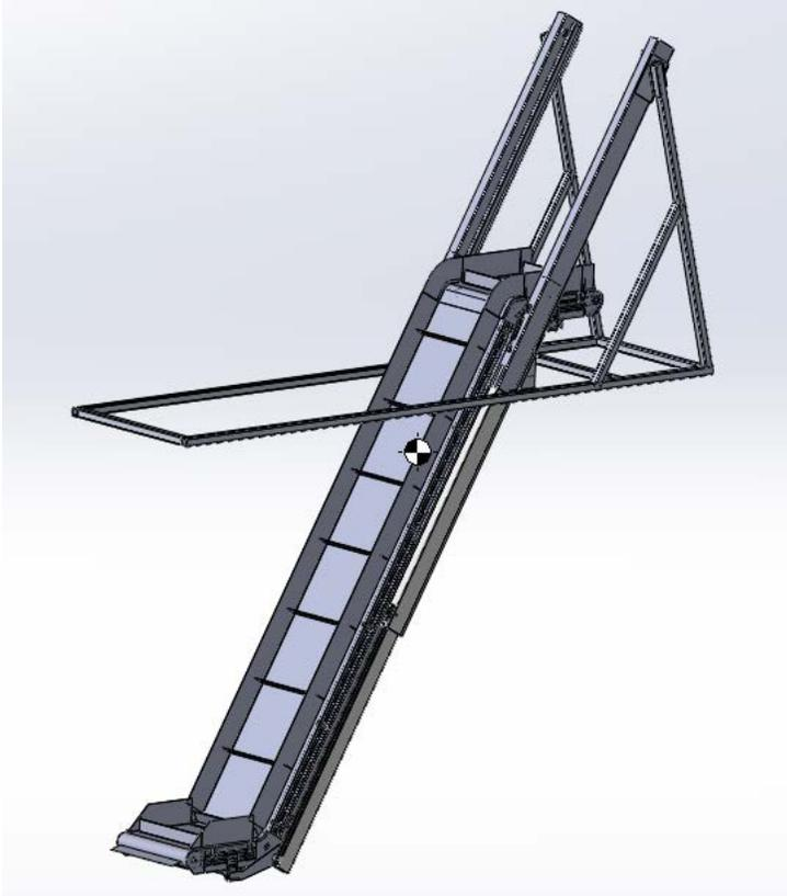
Figure 2.12: Fully assembled and lowered vertical conveyor system
