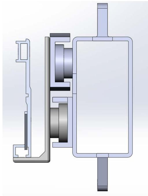
Figure 2.4 Rollers and tracks end view
