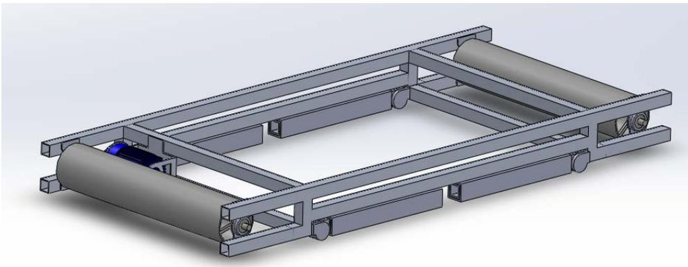
Figure 3.3: Modular conveyor section with legs folded for storage.
