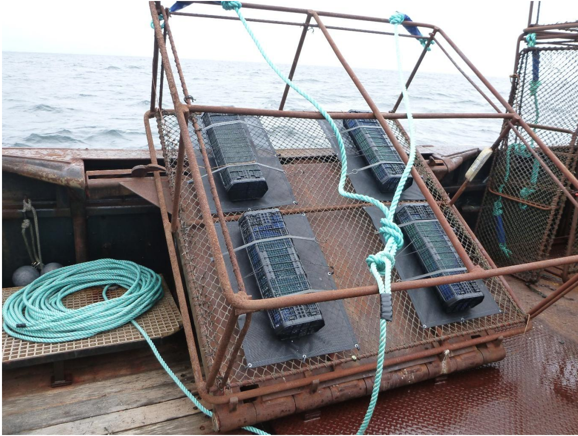
Figure 2. Standard 7 ft x 7 ft, de-netted king crab box pot to be deployed for larval collections and diving operations in 2026. Diver descents/ascents will follow surface marker buoys and lines. Pot steel and bottom netting will serve as diver buoyancy and navigational aids.
